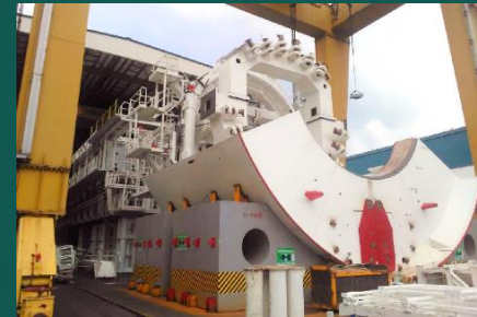
TBM shield under construction
