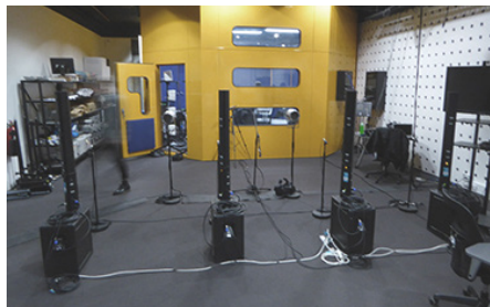
Figure 9: Testing transformation in open environment. Note cancellation equipment in open doorway.
