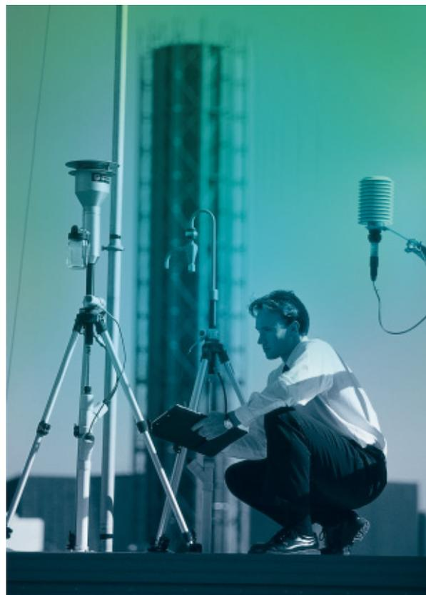
*Monitoring air quality adjacent to the Domain Tunnel vent stack.*
